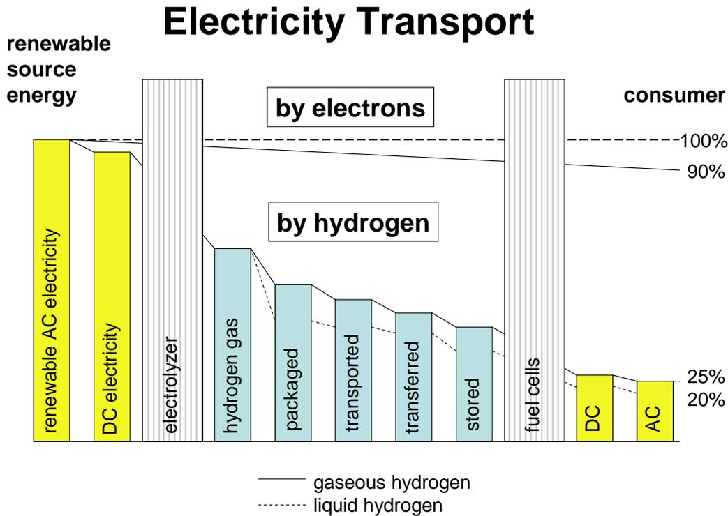
Fig. 15: Energy losses with hydrogen and with direct current from a renewable energy source to the consumer. Source: Bossel 2004 [27]
