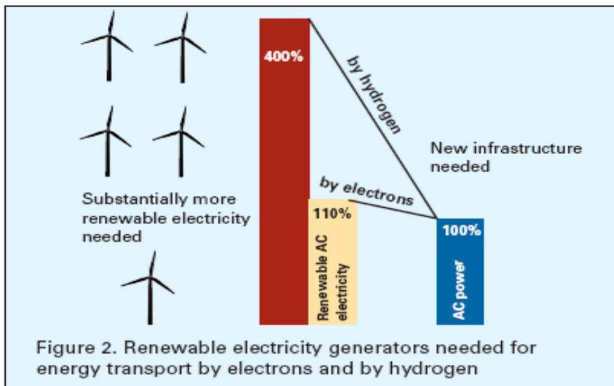
Figure 17 Efficiency of renewable primary sources like wind, solar, hydro; grid transport compared with hydrogen conversion [27]
