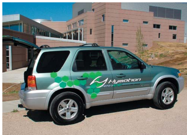
Plug-in hybrids such as this Ford Escape HEV developed by Hymotion are important, not only because of the potential impact this technology can have on reducing gasoline consumption, but also because they can help enable intermittent renewable energy technologies like wind by providing battery storage for electricity from the grid.
