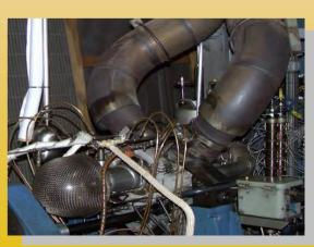
Even moderate fractions of FT fuel blended in JP-8 significantly reduce exhaust emission particulates in T63 turbine engine testing.
