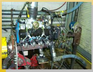
FT fuel burns more completely and emissions are significantly cleaner than EPA certified low-sulfur diesel fuel tested in 6.5L diesel engine.
